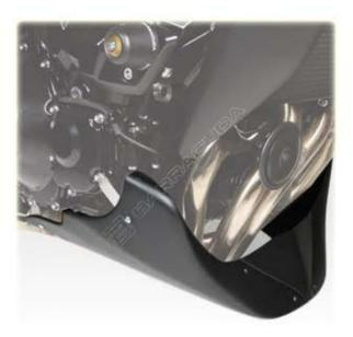
FIX THE ABS ENGINE SPOILER WITH ITS SCREWS KIT 4X10, WASHERS AND NUTS.
